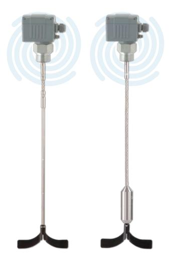
The reliable and maintenance free level limit switch for bulk goods DF11 can be used as full, empty and demand indicator for simple applications. These limit switches are observing the filling level in silos, containers, weighers, discharge pipes etc. and are excellently qualified for use in dusty, powdery, granulated as well as in granular bulk materials.
