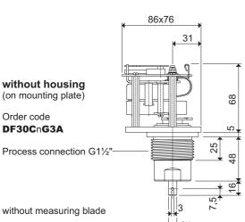
The compact DF30 fits in every discharge taper! We deliver any form of measuring blade as per your request. rotation speed of measuring blade optional in 5 or 8 rpm. (short response times)
